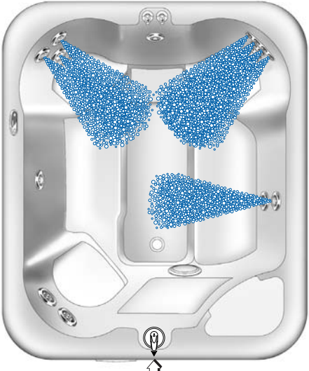
Jet System 4 SmartJet® lever in the 12 o'clock position • 2 stacked directional hydromassage jets on right wall • 10 Precision® jets on right rear • 3 Jet-Cluster™ system on left rear (2 dual port rotary, 1 directional hydromassage)
