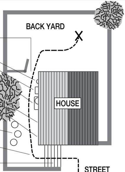
It may be necessary to remove a gate, part of a fence, or other movable obstructions in order to roll the spa to its installation site. About ten percent of the time, a crane is the only way to install the spa by lifting it to its final destination.
