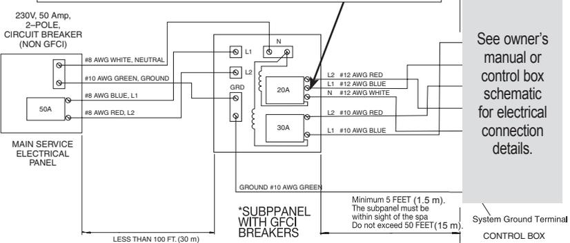
NOTE: The wire connections to GFCI breakers are for reference only. Always ensure the white neutral wire is connected to the load neutral of the 20 amp breaker.
