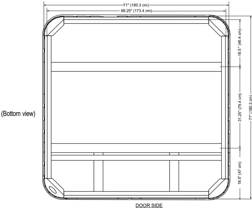
**NOTE: WATKINS WELLNESS** recommends that the SX be installed on a minimum 4" (10.2cm) thick reinforced concrete pad or structurally sound deck able to support the "dead weight" found in the spa specification chart.
