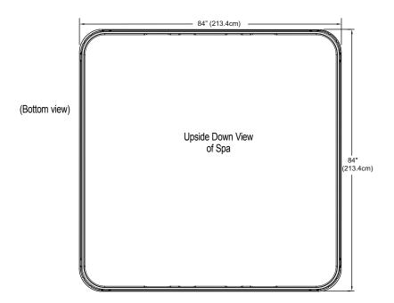
**NOTE:** Watkins Manufacturing Corporation recommends that the Flair be installed on a minimum 4" (10 cm) thick reinforced concrete pad or structurally sound deck able to support the "dead weight" found in the spa specification chart.
