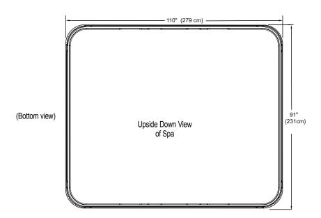
**NOTE:** Watkins Manufacturing Corporation recommends that the Gleam be installed on a minimum 4" (10 cm) thick reinforced concrete pad or structurally sound deck able to support the "dead weight" found in the spa specification chart.
