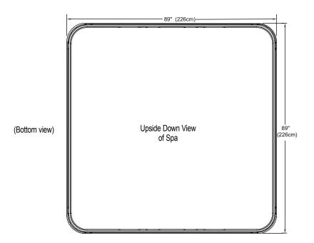
**NOTE:** Watkins Manufacturing Corporation recommends that the Pulse be installed on a minimum 4" (10 cm) thick reinforced concrete pad or structurally sound deck able to support the "dead weight" found in the spa specification chart.
