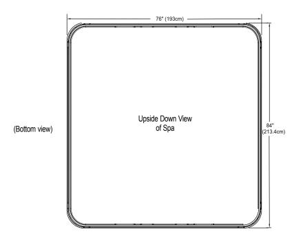
**NOTE:** Watkins Manufacturing Corporation recommends that the Glow be installed on a minimum 4" (10 cm) thick reinforced concrete pad or structurally sound deck able to support the "dead weight" found in the spa specification chart.
