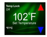
**IMPORTANT:** The red Temperature/Spa lock icon will be lit during a temperature lock condition.
