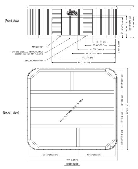
**NOTE:** Watkins Manufacturing Corporation requires that the Landmark be installed on a minimum 4" thick reinforced concrete pad.
