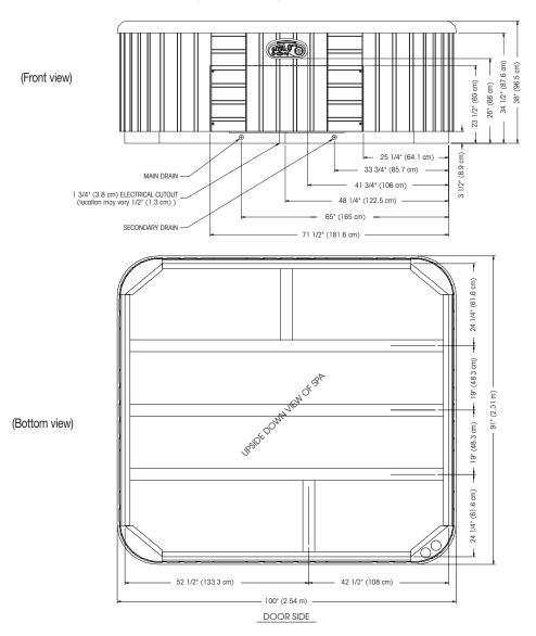
**NOTE:** Watkins Manufacturing Corporation requires that the Landmark® be installed on a minimum 4" thick reinforced concrete pad.
