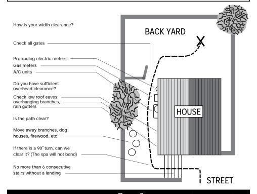
It may be necessary to remove a gate, part of a fence, or other movable obstructions in order to roll the spa to its installation site. About ten percent of the time, a crane is the only way to install the spa by lifting it to its final destination.
