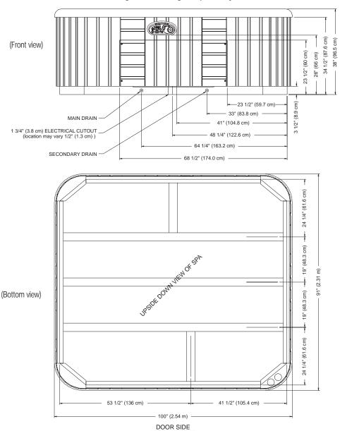
**NOTE:** Watkins Manufacturing Corporation requires that the Grandee be installed on a minimum 4" thick reinforced concrete pad.
