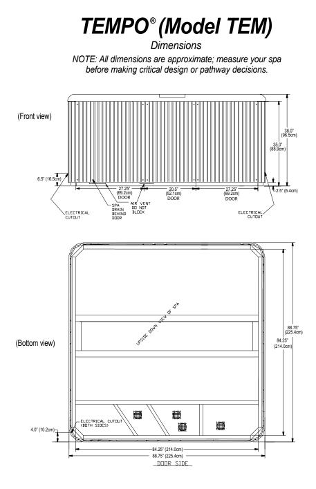
**NOTE:** Watkins Manufacturing Corporation recommends that the Tempo be installed on a minimum 4" (10.2cm) thick reinforced concrete pad or structurally sound deck able to support the "dead weight" found in the spa specification chart.
