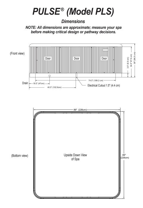
**NOTE:** Watkins Manufacturing Corporation recommends that the Pulse be installed on a minimum 4" thick reinforced concrete pad or structurally sound deck able to support the "dead weight" found in the spa specification chart. **WARNING: The Pulse must not be shimmed in any manner.**
