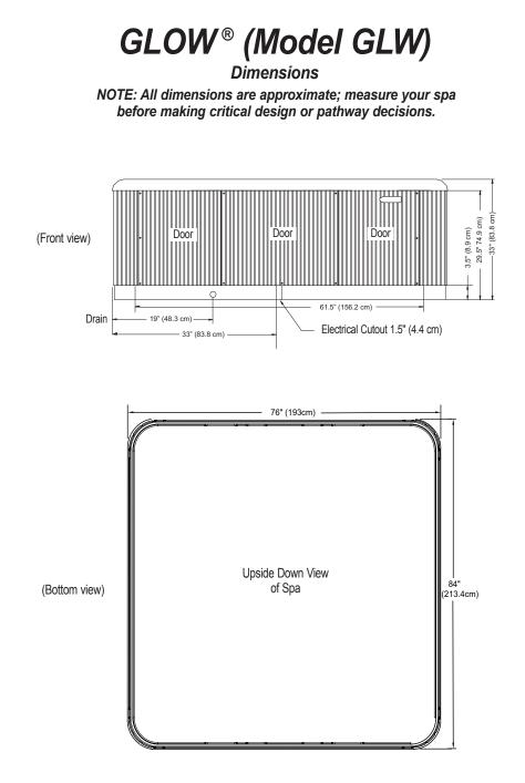
**NOTE:** Watkins Manufacturing Corporation recommends that the Glow be installed on a minimum 4" thick reinforced concrete pad or structurally sound deck able to support the "dead weight" found in the spa specification chart. **WARNING: The Glow must not be shimmed in any manner.**
