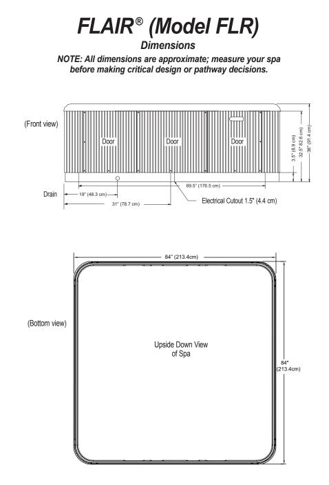
**NOTE:** Watkins Manufacturing Corporation recommends that the Flair be installed on a minimum 4" thick reinforced concrete pad or structurally sound deck able to support the "dead weight" found in the spa specification chart. **WARNING: The Flair must not be shimmed in any manner.**
