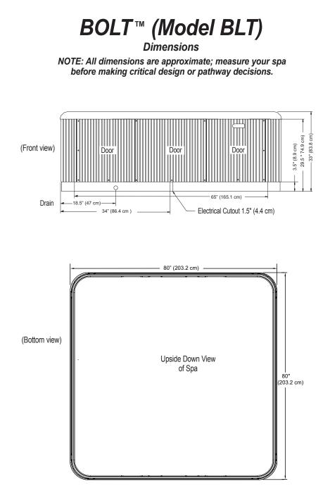
**NOTE:** Watkins Manufacturing Corporation recommends that the Bolt be installed on a minimum 4" thick reinforced concrete pad or structurally sound deck able to support the "dead weight" found in the spa specification chart. **WARNING: The Bolt must not be shimmed in any manner.**
