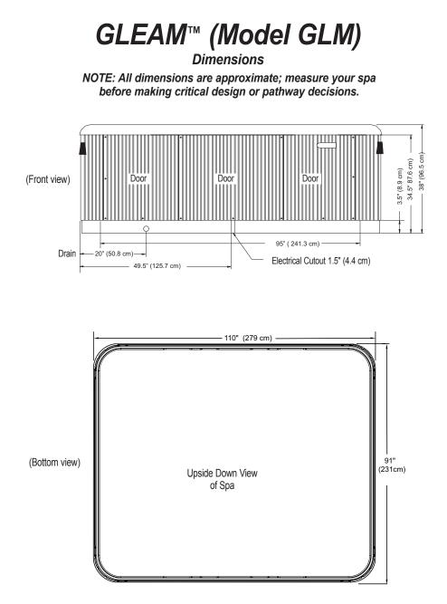
**NOTE:** Watkins Manufacturing Corporation recommends that the Gleam be installed on a minimum 4" thick reinforced concrete pad or structurally sound deck able to support the "dead weight" found in the spa specification chart. **WARNING: The Gleam must not be shimmed in any manner.**
