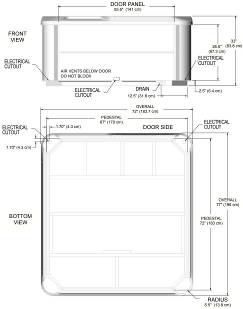
**NOTE: WATKINS WELLNESS** recommends that the SX be installed on a minimum 4" (10.2 cm) thick reinforced concrete pad or structurally sound deck able to support the "dead weight" found in the spa specification chart.
