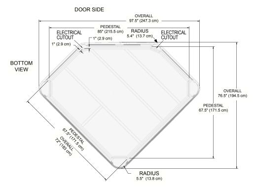
**NOTE: WATKINS WELLNESS** recommends that the TX be installed on a minimum 4" (10.2 cm) thick reinforced concrete pad or structurally sound deck able to support the "dead weight" found in the spa specification chart. **IMPORTANT:** THE TX MUST NOT BE SHIMMED IN ANY MANNER.
