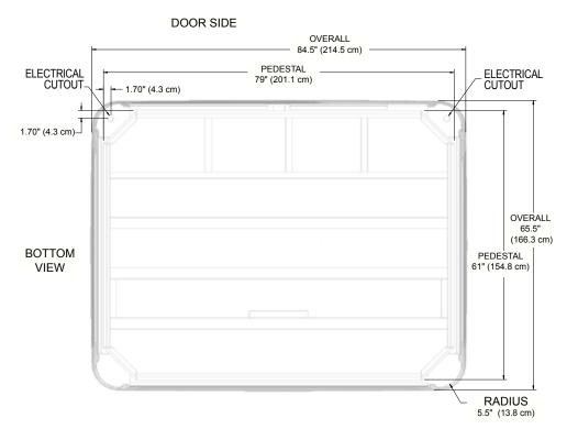
**NOTE: WATKINS WELLNESS** recommends that the STRIDE be installed on a minimum 4" (10.2 cm) thick reinforced concrete pad or structurally sound deck able to support the "dead weight" found in the spa specification chart.
