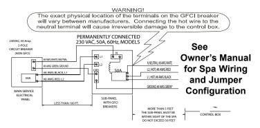
Your electrician should mount the subpanel in the vicinity of the spa but it should not be closer than five feet (1.5 m) from the spa water edge (NEC 680-38 to 41-A-3).
