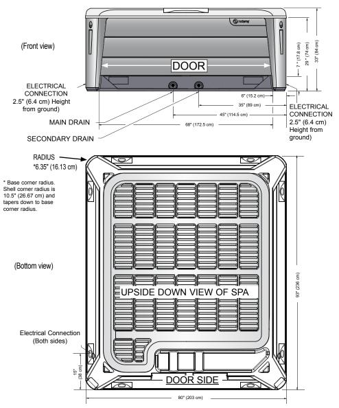
**NOTE: WATKINS WELLNESS** recommends that the **SOVEREIGN** be installed on a minimum 4" (10 cm) thick reinforced concrete pad or a deck that is able to withstand more than 110 lbs/ft<sup>2</sup> (535 kg/m<sup>2</sup>).
