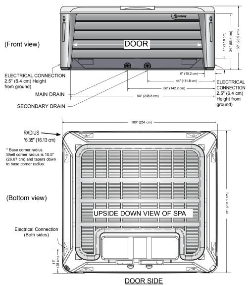
**NOTE: WATKINS WELLNESS** requires that the **GRANDEE** be installed on a minimum 4" (10 cm) thick reinforced concrete pad or a deck that is able to withstand more than 115 lbs/ft<sup>2</sup> (555 kg/m<sup>2</sup>). **WARNING:** The **GRANDEE** must not be shimmed in any manner.
