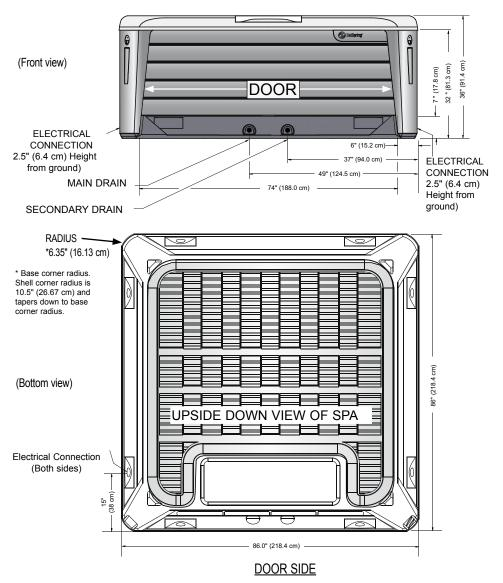
**NOTE: WATKINS WELLNESS** recommends that the **VANGUARD & ARIA** be installed on a minimum 4" (10 cm) thick reinforced concrete pad or a deck that is able to withstand more than 115 lbs/ft<sup>2</sup> (565 kg/m<sup>2</sup>) & 110 lbs/ft<sup>2</sup> (535 kg/m<sup>2</sup>).
