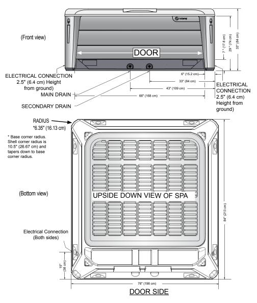
**NOTE: WATKINS WELLNESS** recommends that the **PRODIGY** be installed on a minimum 4" (10 cm) thick reinforced concrete pad or a deck that is able to withstand more than 110 lbs/ft<sup>2</sup> (535 kg/m<sup>2</sup>).
