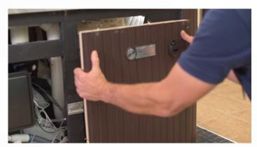
1. Remove the equipment compartment door located directly below the main control panel on the front of the spa.
