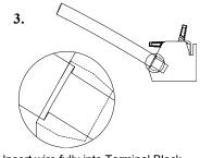
Insert wire fully into Terminal Block
